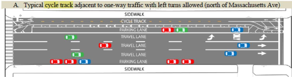
**Figure 27. A typical segment of the 15th Street cycle track in Washington, D.C.**
