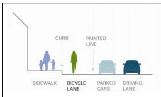
**Figure 5. Cross section view of a street showing bicycle lanes as used in Copenhagen, Denmark.**
