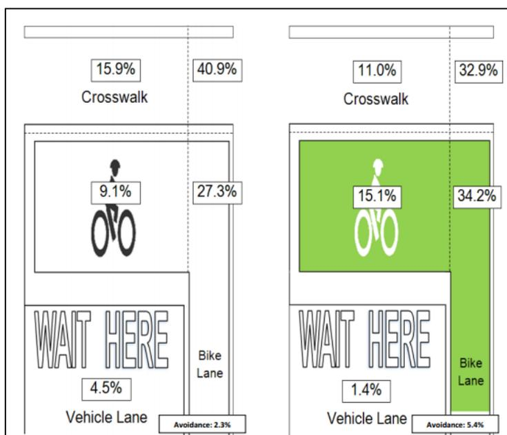
**Figure 34. Stopping location by position from an Austin, Texas bicycle box evaluation.**
