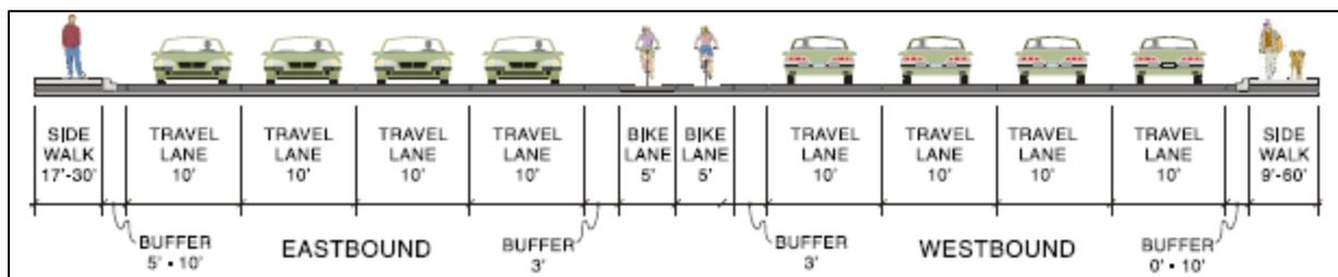
**Figure 17. Cross-section of buffered median bike lanes on Pennsylvania Avenue, Washington, D.C.**
