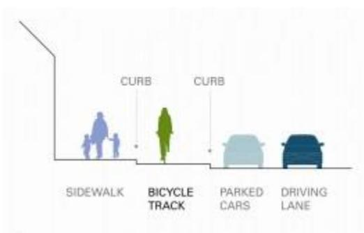
Figure 21. Cross section view of a street showing Copenhagen-style cycle tracks.
