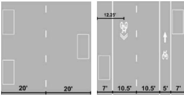
**Figure 60. The reconfiguration of Fremont Street in Seattle, Washington.**
